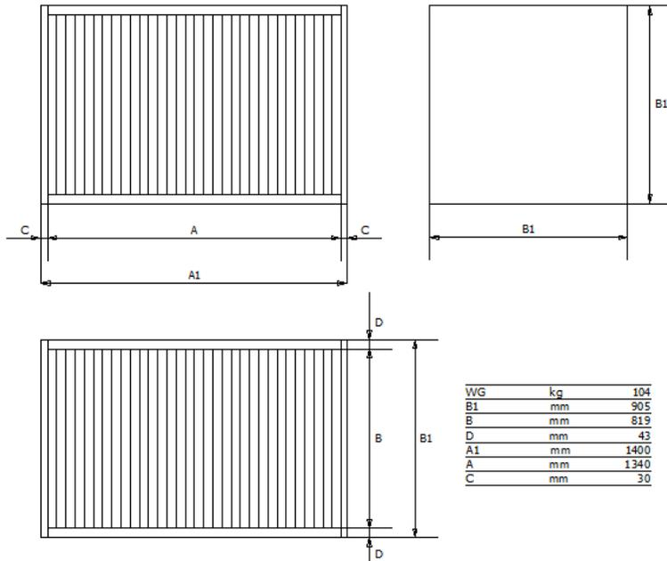
Figure 3: Geometric characteristics of the class H3 heat exchanger used in the analysis (§4.1, §4.2, §3.2).
