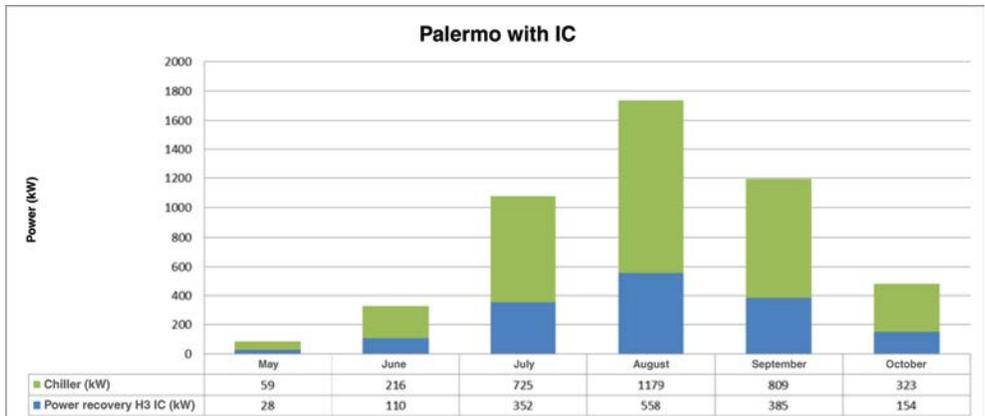
Figure 12: Monthly power draw of powered mechanical ventilation system, and power recovered with class H3 heat exchanger equipped with evaporative cooling, Palermo.
