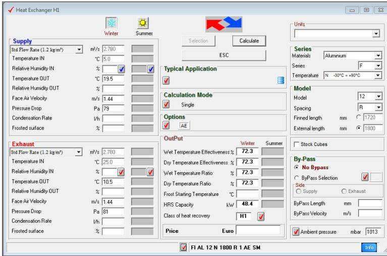
Figure 14: Screenshot of class H1 heat exchanger selection software (§4.3).
