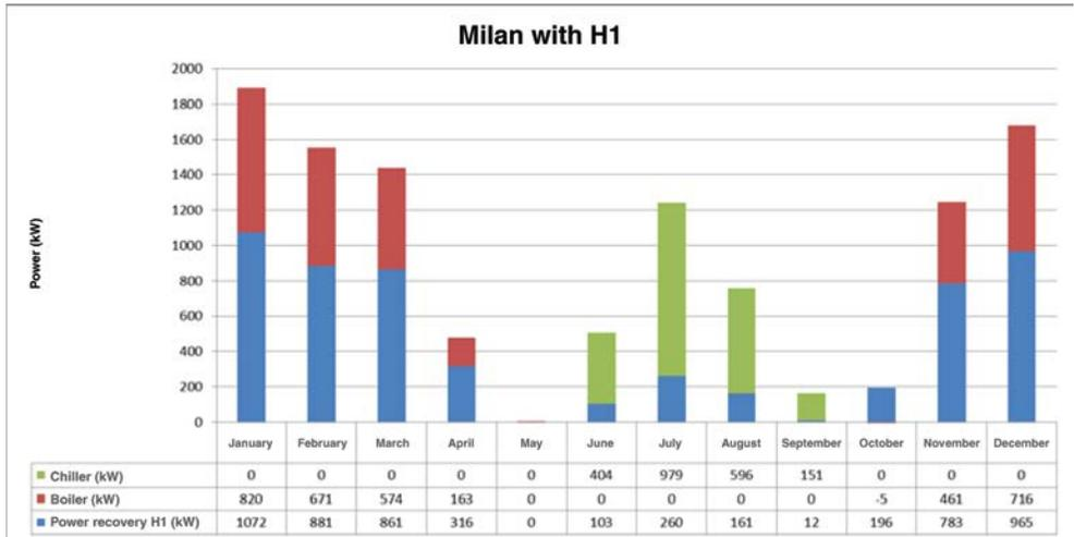
Figure 16: Monthly power draw of powered mechanical ventilation system, and power recovered with class H1 heat exchanger, Milan.
