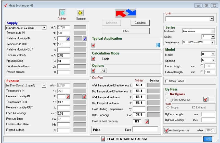
Figure 4: Screenshot of class H3 heat exchanger selection software (§4.1, §4.2).
