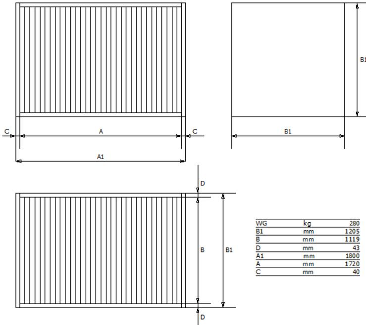
Figure 15: Geometrical characteristics of the class H1 heat recovery unit used in the analysis (§4.3).
