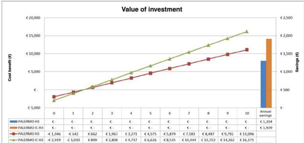
Figure 13: Cost benefits of class H3 recovery unit, with and without evaporative cooling (IC), Palermo.
