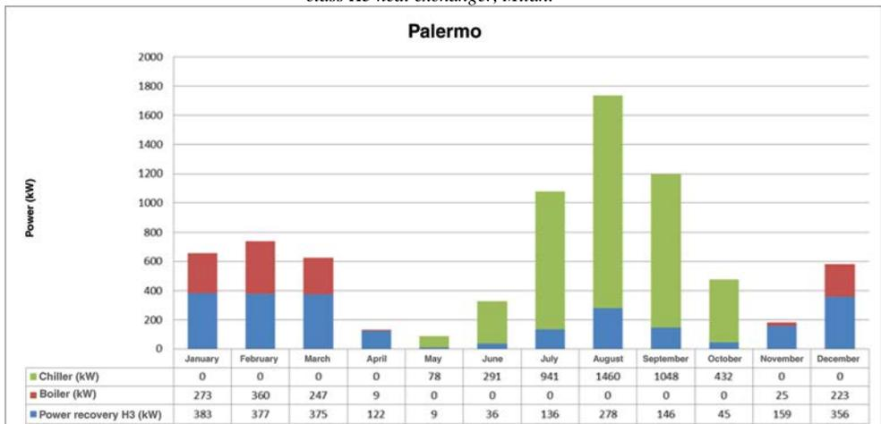
Figure 9: Monthly power draw of powered mechanical ventilation system, and power recovered with class H3 heat exchanger, Palermo.
