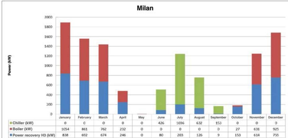
Figure 8: Monthly power draw of powered mechanical ventilation system, and power recovered with class H3 heat exchanger, Milan.
