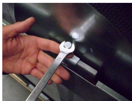
3) Adjust convergence of the wheel using the vertical screw (screw 2)
