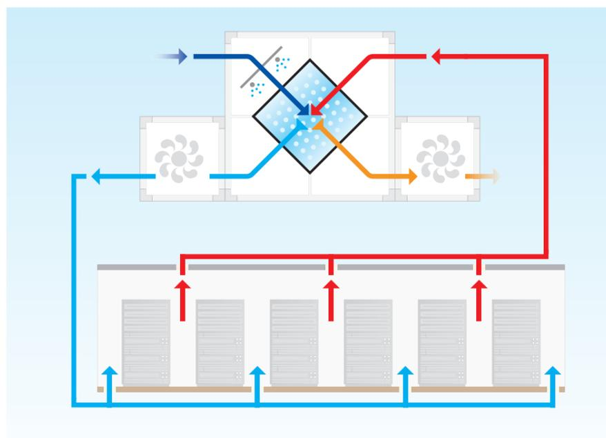
In this application the system is arranged in recirculation mode: the primary air is extracted from the data center, cooled down through the plate heat exchanger in adiabatic mode and finally it is supplied back to the facility.
