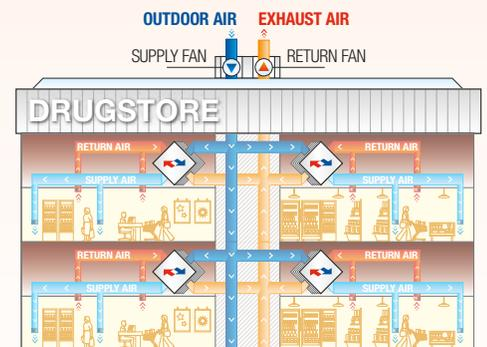
The air quality in a building is one of the main factors for internal comfort. The air must be continuously changed to maintain safe conditions. This process wastes energy, which can be recovered by installing a plate heat exchanger. Let's examine a drugstore with an area of 1235 m<sup>2</sup>, and an average density of 310 people. To change the air, 10,000 m<sup>3</sup>/h of fresh air, is needed. The example shows a system with our air to air plate heat exchanger:
